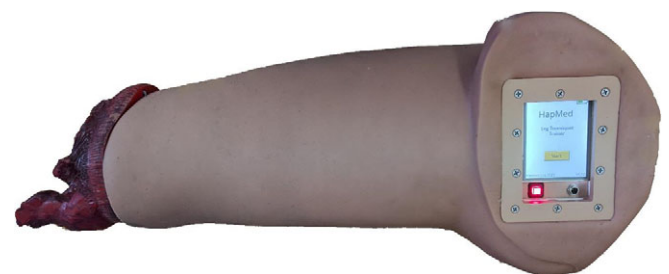
FIGURE 3. The HapMed Leg Tourniquet Trainer (CHI Systems, Fort Washington, PA) simulates an amputation injury proximal to the knee. The trainer contains a computer with touch screen and is operated according to input entered by the operator. The trainer senses pressure applied by a tourniquet and can provide feedback accordingly.
